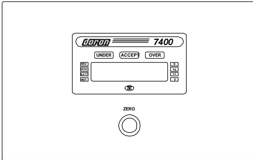
**Figure 1. 7400 Front Panel Layout**
